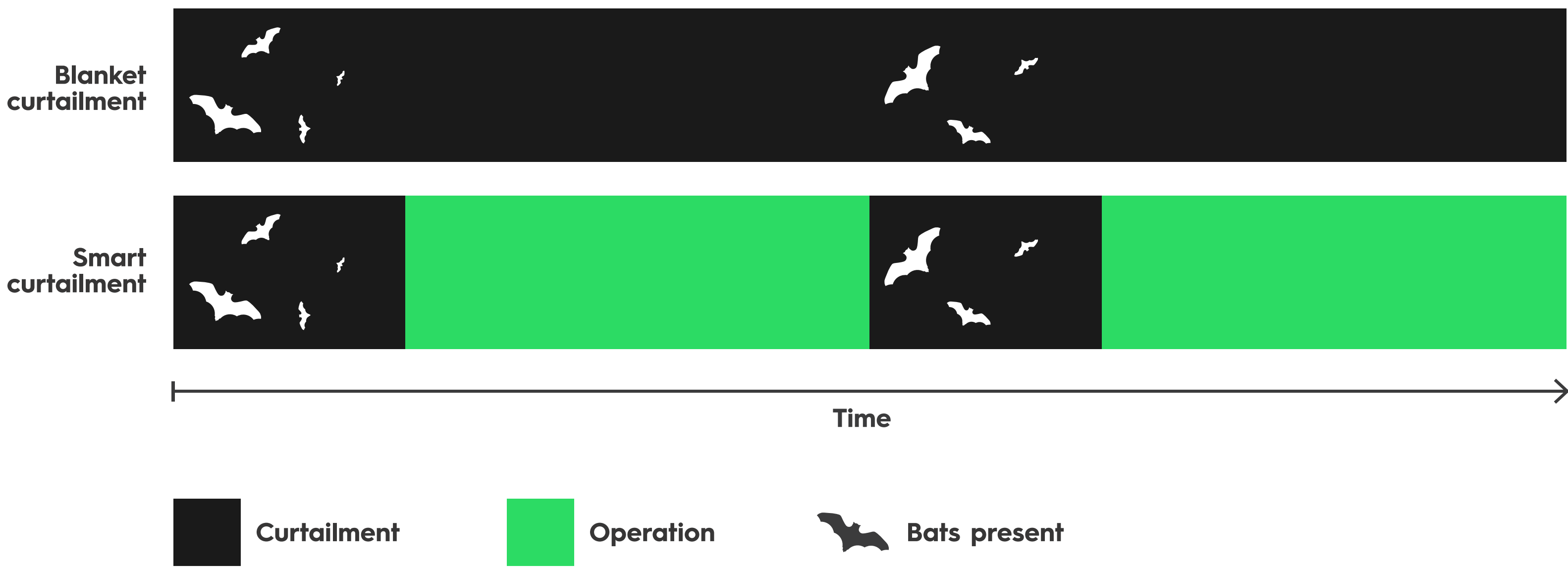
FIGURE 2: Comparison between blanket and smart curtailment strategies for the same wind speed within a given time period.
